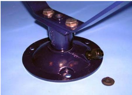
**5.** Remove the Blanking Plug from the Bellows Bottom Bush.
