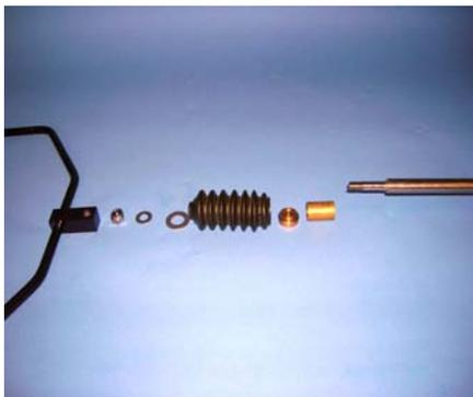
4. When installing the Under Deck mechanism, first separate the following items. U-Piece Assembly, M8 nyloc nut, M8 plain washer, M12 plain washer, Rubber Bellows, Bellows Top Bush and the Push Rod Top Bush
