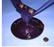
Remove the blanking plug from the bellows bottom bush.
