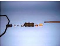
When installing the under deck Mechanism first separate the following items. u-piece assembly, M8 nyloc nut, M8 plain washer, M12 plain washer, rubber
