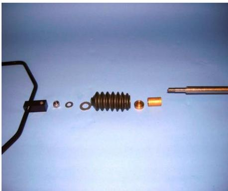
4. When installing the Under Deck mechanism, first separate the following items. U-Piece Assembly, M8 nyloc nut, M8 plain washer, M12 plain washer, Rubber Bellows, Bellows Top Bush and the Push Rod Top Bush
