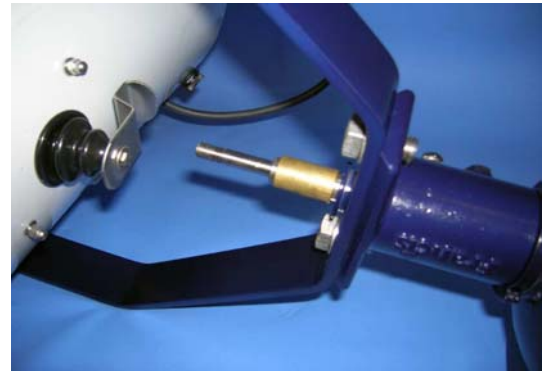
8. Re-Fit the following items: Push Rod Top Bush
